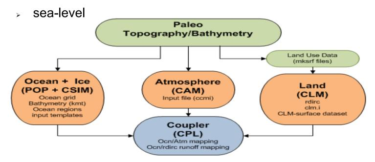
Schematic of PaleoCCSM3 initial and forcing files. Green boxes represent user-provided topography, bathymetry, and land use files. Orange and blue boxes represent files generated using setup tools and guidance outlined in this document.
